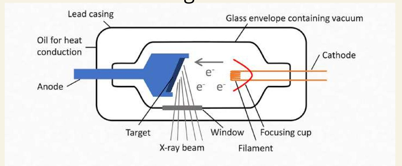
8) This is because electrons are attracted to the anode that has a positive charge.
