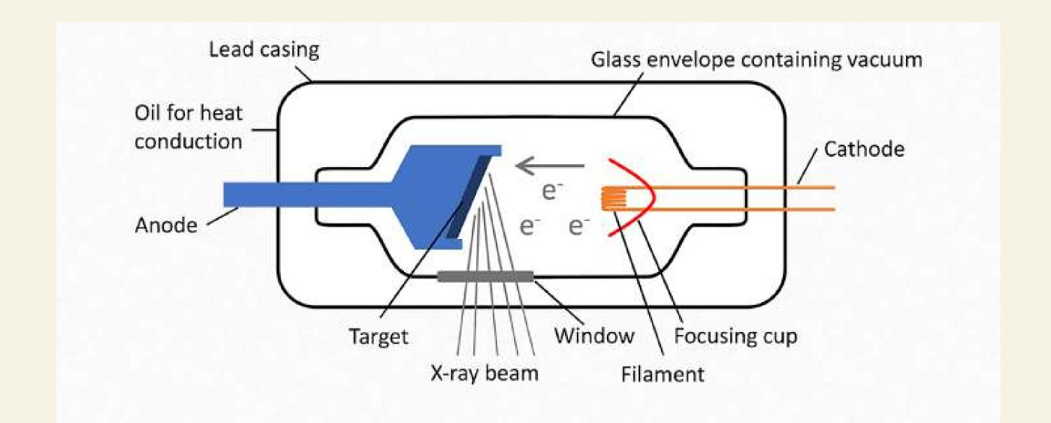
7) With high voltage and energy, these electrons move fast and they start to hit or collide with the metal target.
