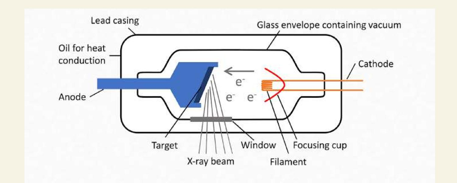
9) X-ray are formed when the bombarding electrons slow down. This is called braking radiation.
