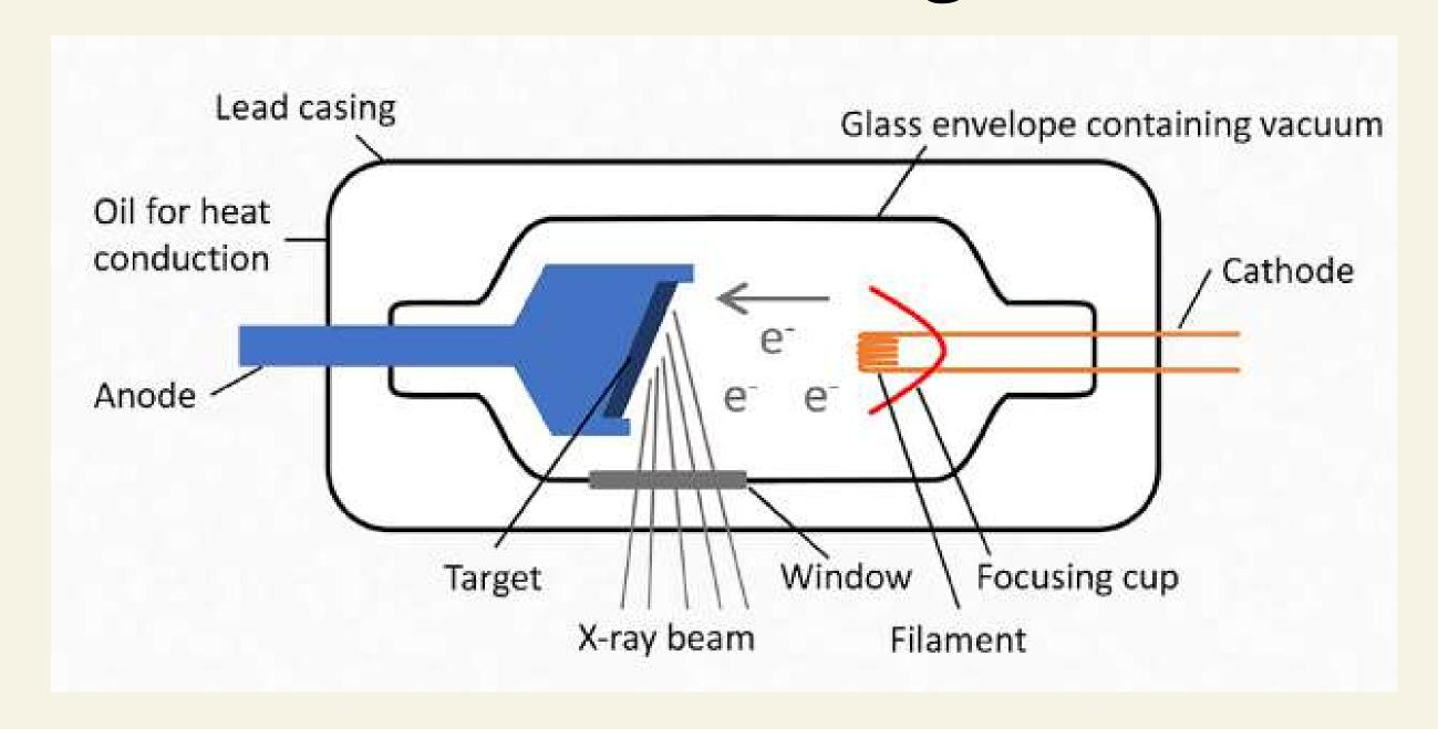
2) To start the process, it needs to heat up as current passes through.
